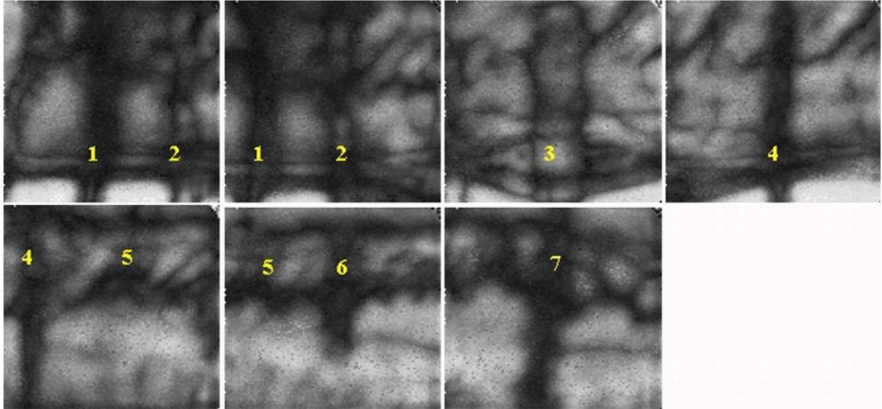
**Figure 9.** A series of C-scan images for the foreign objects contained in the porcine tissue sample. The bold numbers indicate the specific foreign object according to Table 1.
