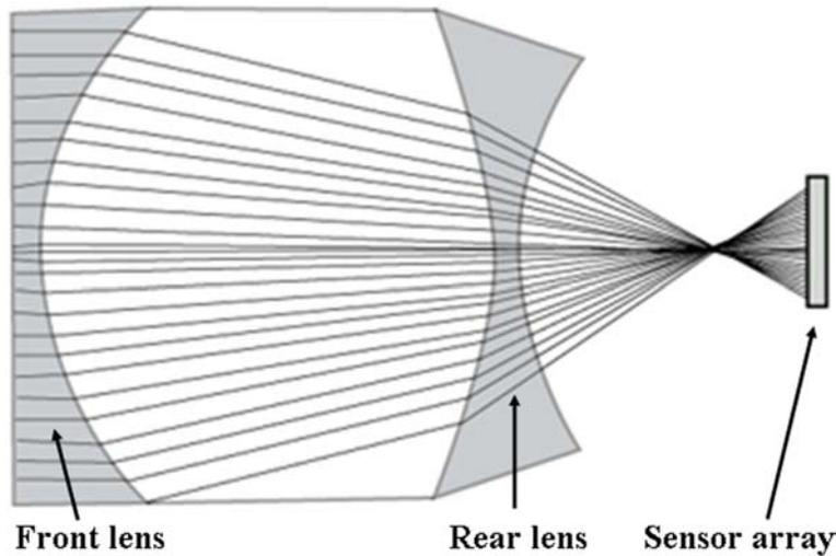
Figure 3. A diagram showing ray tracing of the ultrasound with the compound lens when a parallel beam is used.
