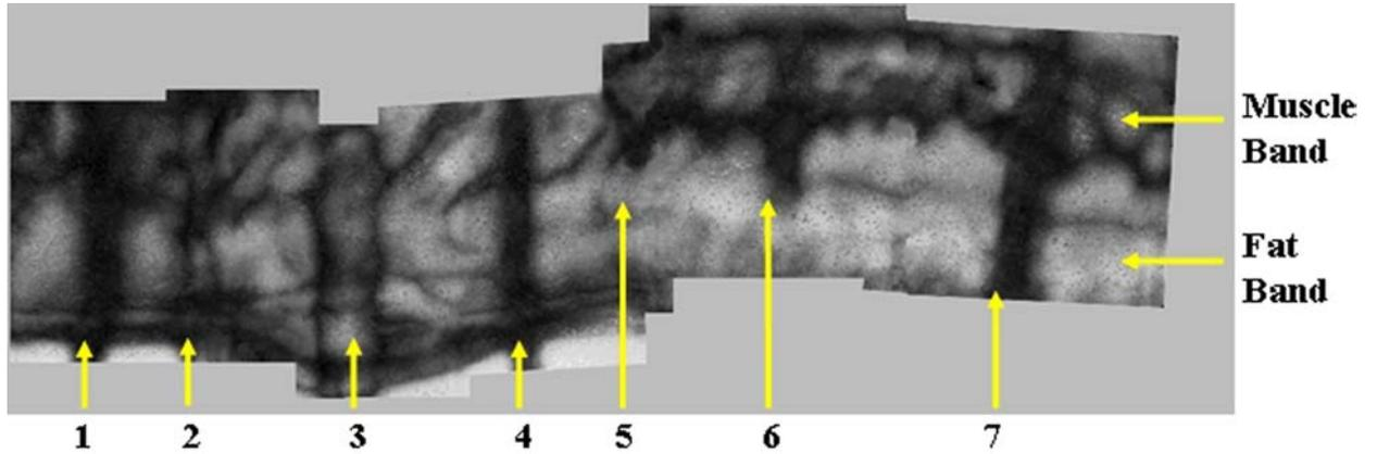
**Figure 10.** The stitched C-scan image of the porcine tissue sample containing the foreign objects. The arrows point to the locations of the foreign objects inserted in the porcine tissue and the numbers indicate the foreign objects according to Table 1.
