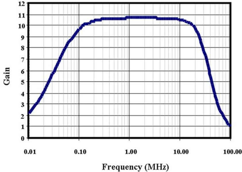
Figure 2. The frequency responsive range of this array.
