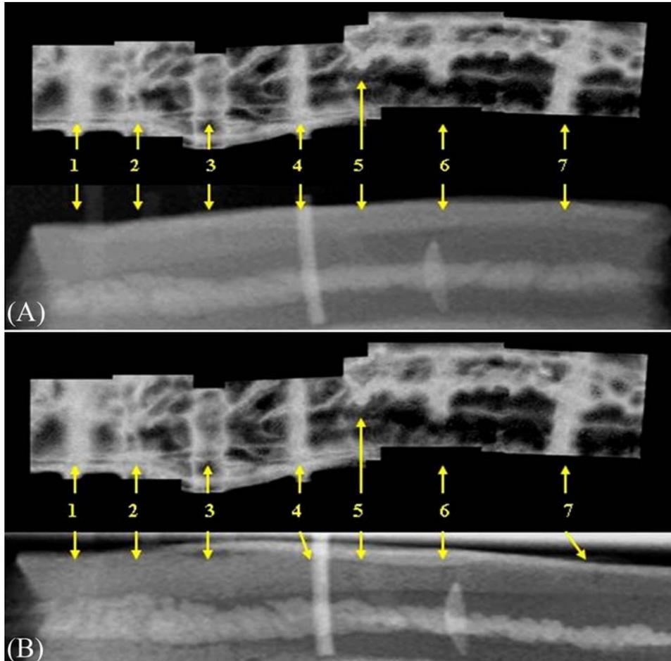
**Figure 13.** Displays of the inverted C-scan image with film-based radiograph and CR image: (A) C-scan image vs. film-based radiograph and (B) C-scan image vs. CR image. The numbers indicate the foreign objects corresponding to Table 1.
