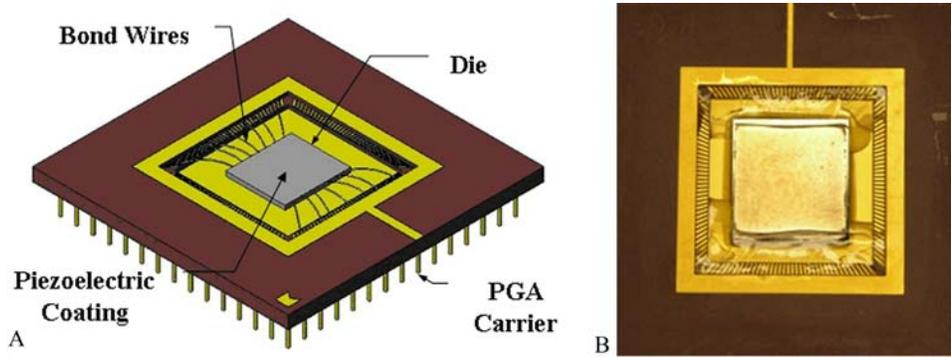
**Figure 1.** (a) Diagram of the PE-CMOS sensor array. (b) A photograph of the chip.
