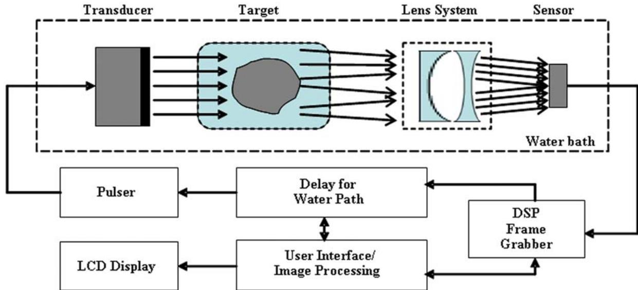
**Figure 4.** Schematic diagram of the C-scan ultrasound imaging geometry.
