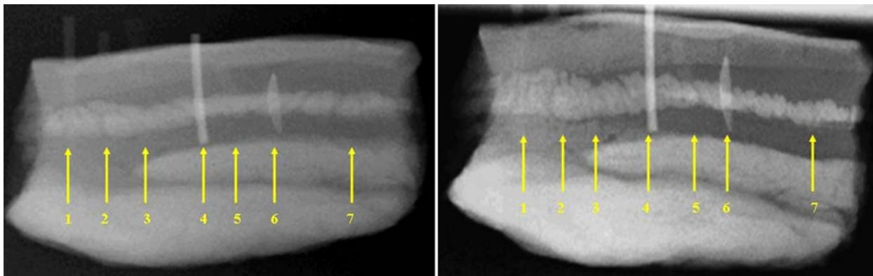
**Figure 12.** (A) The film-based radiograph obtained at 44kVP. (B) The CR image obtained at 40kVP. The arrows point to the locations of the foreign objects inserted in the porcine tissue. The numbers indicate the foreign objects corresponding to Table 1.
