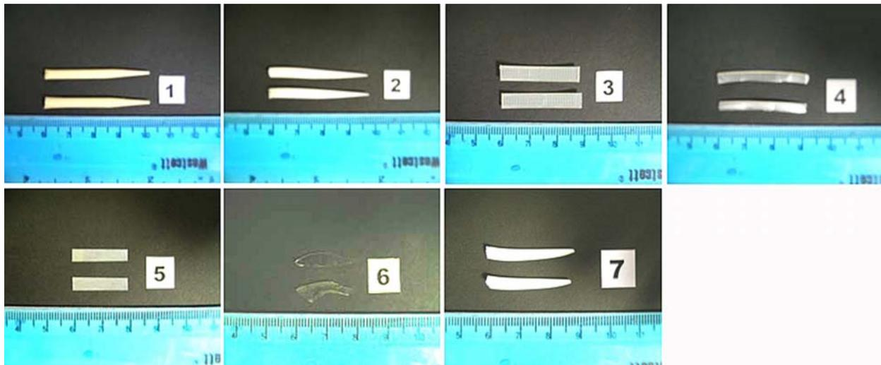
**Figure 7.** The foreign objects used in the experiment: objects of No.1 are bamboo skewers; Nos. 2, 3, and 7 are plastic sticks; Nos. 4 and 5 are aluminum alloys; No.6 are pieces of glass. Note that only one object in each category was selected.
