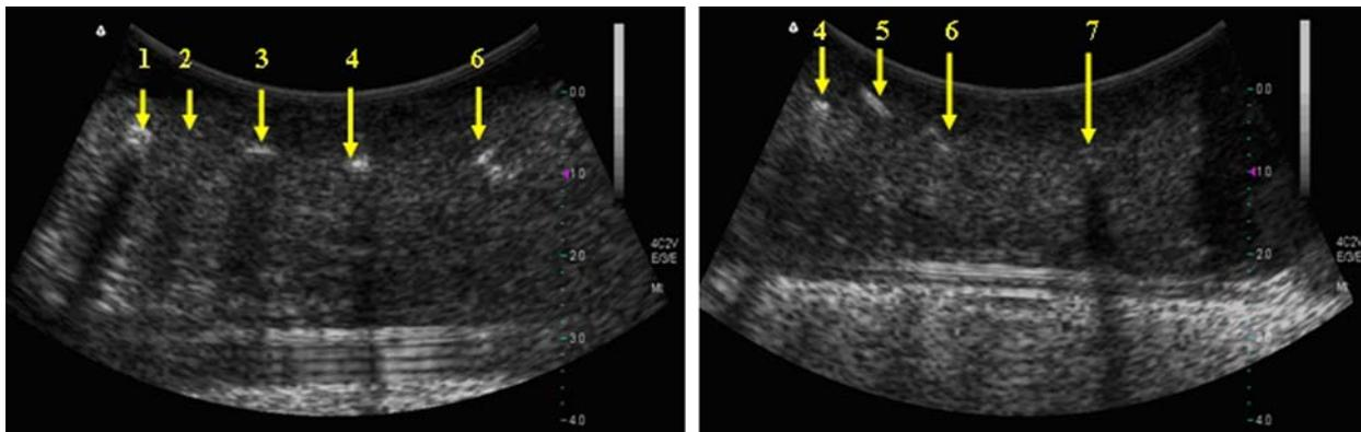
**Figure 11.** The B-scan ultrasound images of the porcine tissue with foreign objects. The arrows point to the locations of the foreign objects inserted in the porcine tissue. The numbers indicate the foreign objects and correspond to Table 1.
