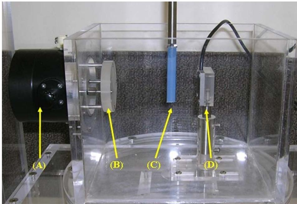
**Figure 5.** A photograph of the of the C-scan prototype. Arrows represents the locations of major components of the prototype (left to right): (A) the sensor unit is directly mounted on the left side of the water tank, (B) acoustic lens system, (C) the imaging target, and (D) the plane-wave transducer.
