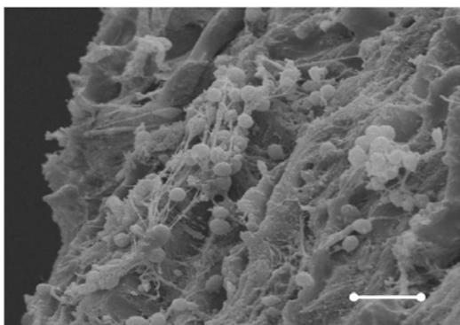
**Figure 2.** Scanning electron microscopy of PLGA scaffold seeded with human embryonic stem cells. Fabrication techniques enable the manufacture of scaffolds to the desired size. The pore sizes in this scaffold are 125 – 250 µm.
